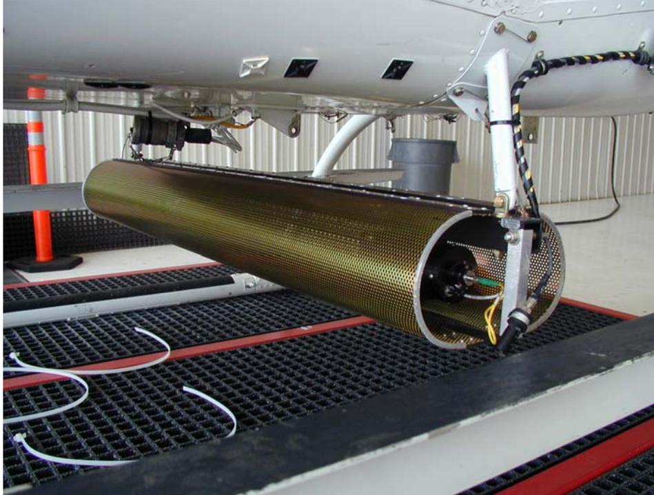
**Figure 3.** The Boreal laser sensor cell, without cover.
